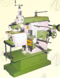
UNIVERSAL - 12" STROKE GEARED/BELT DRIVE
